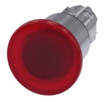
Illuminated mushroom pushbutton, 22 mm, round, metal, shiny, red, 40 mm, 3 switch positions, after pushing in Retraction to center position, after pulling out the button Retraction to center position, with laser labeling, lower case
