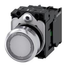
Illuminated pushbutton, 22 mm, round, Metal, shiny, transparent, pushbutton, flat, momentary contact type, with holder, 1NO, LED module with integrated LED 230 V AC, screw terminal, with laser labeling, symbol number according to, ISO 7000 or IEC 60417
