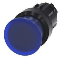
Illuminated mushroom pushbutton, 22 mm, round, plastic, blue, 30 mm, momentary contact type, with laser labeling, upper case and lower case, always upper case at the beginning of the word
