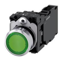
Illuminated pushbutton, 22 mm, round, metal, shiny, green, pushbutton, flat, momentary contact type, with holder, 1 NO+1 NC, LED module with integrated LED 110 V AC, screw terminal, with laser labeling, symbol number according to, ISO 7000 or IEC 60417
