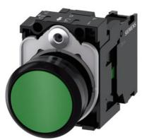
Pushbutton, 22 mm, round, plastic, green, pushbutton, flat, momentary contact type, with holder 1 NO, screw terminal, Z=20-unit packaging
