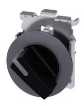
Illuminable selector switch, 30 mm, round, Metal matt, black, Selector switch short, front ring for flush installation, latching, actuating angle 90°, 10:30 /13:30, Z=50-unit packaging
