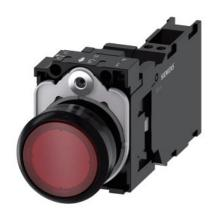
Illuminated pushbutton, 22 mm, round, plastic, red, pushbutton, flat, momentary contact type, with holder, 1 NO+1 NC, LED module with integrated LED 24 V AC/DC, spring-type terminal, with laser labeling, inscription or symbol Customer-specific selection with SIRIUS ACT configurator (CIN)
