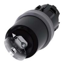
Key-operated switch IKON, 22 mm, round, plastic with metal front ring, lock number 360012K1, with 2 keys, 2 switch positions O<I, momentary contact type, Actuating angle 45°, 10:30h/12h, key removal O, with laser labeling, upper case and lower case, always upper case at the beginning of the word
