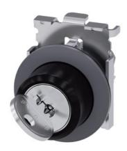
RONIS key-operated switch, 30 mm, round, Metal, matte, front ring for flush installation, lock number SB30, with 2 keys, 2 switch positions O<I, momentary contact type, Actuating angle 45°, 10:30h/12h, key removal O, possible special locks: SB31, 421, 455, with laser labeling, lower case
