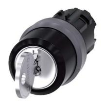
RONIS key-operated switch, 22 mm, round, plastic with metal front ring, lock number 455, with 2 keys, 3 switch positions I-O-II, latching, actuating angle  $2x45^{\circ}$ , 10:30h/12h/13:30h, Key removal I+O+II, with laser labeling, upper case and lower case, always upper case at beginning of line
