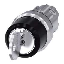
RONIS key-operated switch, 22 mm, round, metal, shiny, lock number SB30, with 2 keys, 3 switch positions I-O-II, latching, actuating angle 2x45°, 10:30h/12h/13:30h, key removal O+I, possible special locks: SB31, 421, 455, with laser labeling, lower case
