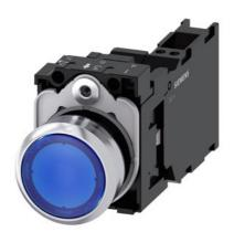
Illuminated pushbutton, 22 mm, round, metal, shiny, blue, pushbutton, flat, momentary contact type, with holder, 1 NO+1 NC, LED module with integrated LED 110 V AC, spring-type terminal, with laser labeling, symbol number according to, ISO 7000 or IEC 60417
