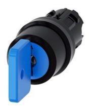
Key-operated switch O.M.R, 22 mm, round, plastic, lock number 73038, blue, with 2 keys, 3 switch positions I-O<II, left latching, right momentary contact type, actuating angle  $2x45^{\circ}$ , 10:30h/12h/13:30h, key removal O, with laser labeling, upper case and lower case,
