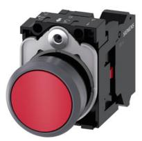
Pushbutton, 22 mm, round, plastic with metal front ring, red, pushbutton, flat, momentary contact type, with holder, 1 NC, spring-type terminal, with laser labeling, symbol number according to, ISO 7000 or IEC 60417
