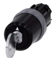
key-operated switch Siemens, 22 mm, round, plastic with metal front ring, lock number SSG10, with 2 keys, 3 switch positions I-O-II, latching, actuating angle 2x45°, 10:30h/12h/13:30h, key removal I+O+II
