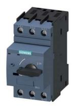
Circuit breaker size S00 for starter combination Rated current 2 A N-release 26 A screw terminal Standard switching capacity
