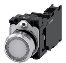
Illuminated pushbutton, 22 mm, round, Metal, shiny, transparent, pushbutton, flat, momentary contact type, with holder, 1 NO+1 NC, LED module with integrated LED 230 V AC, spring-type terminal, with laser labeling, upper case and lower case, always upper case at the beginning of the word
