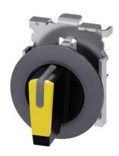
Selector switch, illuminable, 30 mm, round, Metal, matte, yellow, selector switch, short, front ring for flush installation, 3 switch positions I-O-II, latching, actuating angle 2x45°, 10:30h/12h/13:30h, Z=50-unit packaging
