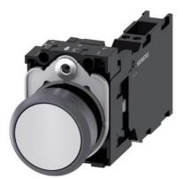
Pushbutton, 22 mm, round, plastic with metal front ring, white, pushbutton, flat, momentary contact type, with holder, 1 NO+1 NC, spring-type terminal, with laser labeling, inscription or symbol Customer-specific selection with SIRIUS ACT configurator (CIN)
