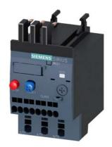
Overload relay 1.8...2.5 A Thermal For motor protection Size S00, Class 10 Contactor mounting Main circuit: Spring-type terminal Auxiliary circuit: spring-type terminal Manual-Automatic-Reset
