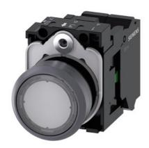
Illuminated pushbutton, 22 mm, round, plastic with metal front ring, clear, pushbutton, flat, momentary contact type, with holder, 1NO, LED module with integrated LED 24 V AC/DC, spring-type terminal, with laser labeling, upper case
