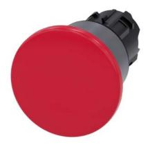
Mushroom pushbutton, 22 mm, round, plastic with metal front ring, red, 40mm, latching, pull-to-unlatch mechanism, Z=50-unit packaging
