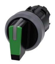
Selector switch, illuminable, 22 mm, round, plastic with metal front ring, green, selector switch, short, 3 switch positions I>O<II, momentary contact type, actuating angle  $2x45^{\circ}$ , 10:30h/12h/13:30h, Z=50-unit packaging
