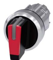
Selector switch, illuminable, 22 mm, round, metal, shiny, red, selector switch, short, 3 switch positions I>O<II, momentary contact type, actuating angle 2x45°, 10:30h/12h/13:30h, Z=50-unit packaging
