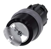
RONIS key-operated switch, 22 mm, round, plastic with metal front ring, lock number 455, with 2 keys, 2 switch positions O<I, momentary contact type, Actuating angle 45°, 10:30h/12h, key removal O, with laser labeling, lower case
