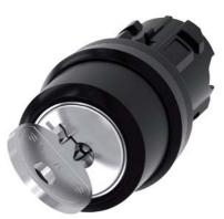
RONIS key-operated switch, 22 mm, round, plastic, lock number 455, with 2 keys, 2 switch positions O-I, latching, actuating angle 90°, 10:30h/13:30h, key removal O+I, with laser labeling, upper case and lower case, always upper case at beginning of line
