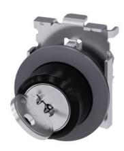
RONIS key-operated switch, 30 mm, round, Metal, matte, front ring for flush installation, lock number SB30, with 2 keys, 2 switch positions O-I, latching, actuating angle 90°, 10:30h/13:30h, key removal I, possible special locks: SB31, 421, 455, with laser labeling, inscription or symbol Customer-specific selection with SIRIUS ACT configurator (CIN)
