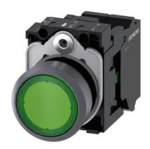
Illuminated pushbutton, 22 mm, round, plastic with metal front ring, green, pushbutton, flat, momentary contact type, with holder, 1NO, LED module with integrated LED 24 V AC/DC, spring-type terminal, with laser labeling, symbol number according to, ISO 7000 or IEC 60417
