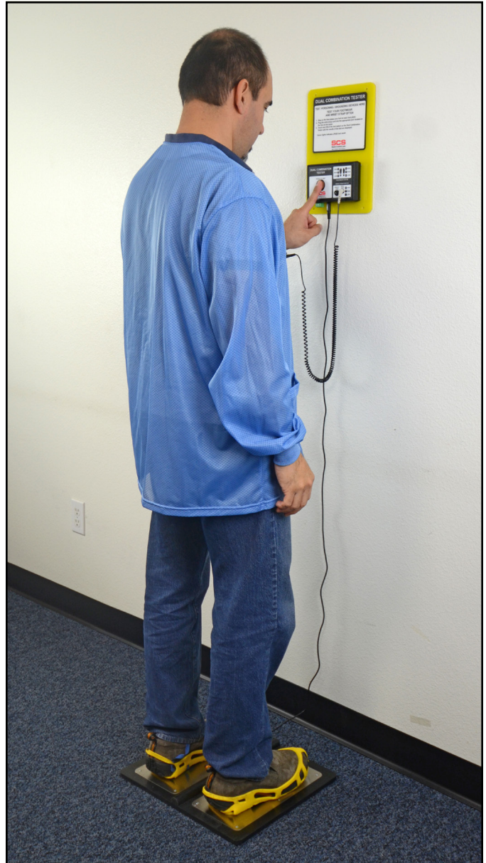
Figure 12. Using the Dual Combination Tester
