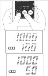
4. Point the plate in the airflow of the ionizer to be measured and press the START button.
