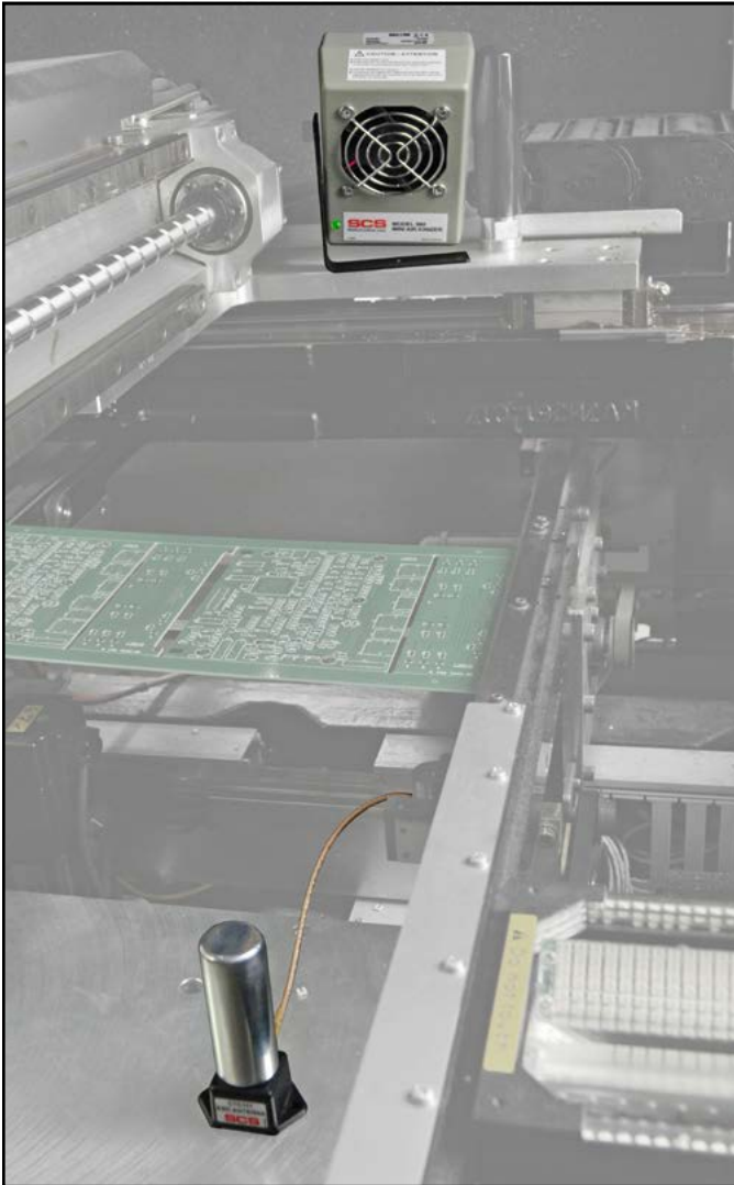
Figure 24. Using the EM Aware Monitor with ionizer antenna inside of a pick-and-place machine with the SCS 960 Mini Air Ionizer
