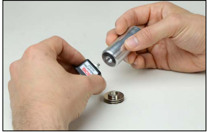
Figure 4. Replacing the standard antenna with the ionizer antenna
