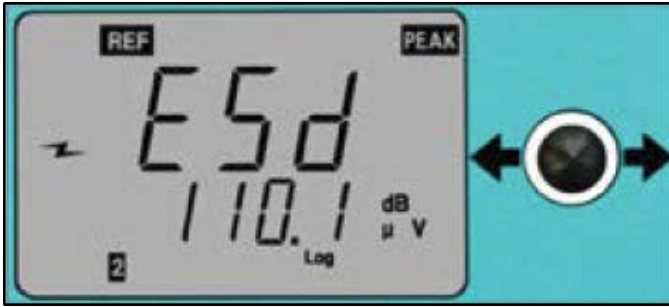
Figure 11. Modifying the ESD event threshold
