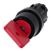
Key-operated switch O.M.R, 22 mm, round, plastic, lock number 73037, red, with 2 keys, 2 switch positions O<I, momentary contact type, Actuating angle 45°, 10:30h/12h, key removal O, with laser labeling, lower case
