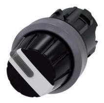
Selector switch, illuminable, 22 mm, round, plastic with metal front ring, white, Rotary knob, 2 switch positions O-I, latching, actuating angle 90°, 10:30h/13:30h, with laser labeling, upper case and lower case, always upper case at beginning of line
