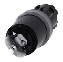
Key-operated switch IKON, 22 mm, round, plastic with metal front ring, lock number 360012K1, with 2 keys, 2 switch positions O-I, latching, actuating angle  $90^\circ$ , 10:30h/13:30h, key removal O+I, with laser labeling, upper case
