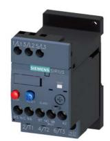
Overload relay 2.2...3.2 A Thermal For motor protection Size S00, Class 10 Stand-alone installation Main circuit: Screw Auxiliary circuit: Screw Manual-Automatic-Reset
