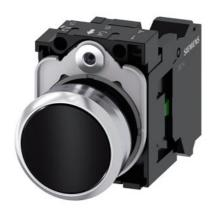
Pushbutton, 22 mm, round, metal, shiny, black, pushbutton, flat, momentary contact type, 1 NO, spring-type terminal, with laser labeling, upper case and lower case, always upper case at beginning of line
