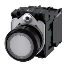
Illuminated pushbutton, 22 mm, round, plastic, clear, pushbutton, flat, momentary contact type, with holder, 1NO, LED module with integrated LED 230 V AC, screw terminal, with laser labeling, inscription or symbol Customer-specific selection with SIRIUS ACT configurator (CIN)
