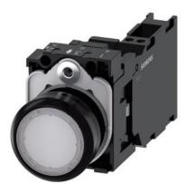
Illuminated pushbutton, 22 mm, round, plastic, white, pushbutton, flat, momentary contact type, with holder, 1 NO+1 NC, LED module with integrated LED 24 V AC/DC, spring-type terminal, with laser labeling, upper case and lower case, always upper case at beginning of line
