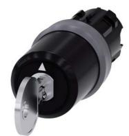
key-operated switch Siemens, 22 mm, round, plastic with metal front ring, special lock, with 2 keys, 3 switch positions I>O<II, momentary contact on the left, latching on the right, actuating angle 2x45°, 10:30h/12h/13:30h, key removal O+II
