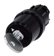
key-operated switch Siemens, 22 mm, round, plastic, lock no. LSG1, with 2 keys, 2 switch positions O<I, momentary contact type, actuating angle 45°, 10:30h/12h, key removal O, with laser labeling, inscription or symbol customer-specific selection with SIRIUS ACT configurator (CIN)
