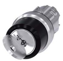
RONIS key-operated switch, 22 mm, round, metal, shiny, lock number 455, with 2 keys, 2 switch positions O-I, latching, actuating angle 90°, 10:30h/13:30h, key removal O+I, with laser labeling, lower case
