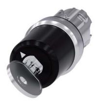
Key-operated switch BKS, 22 mm, round, metal, shiny, lock number S1, with 2 keys, 2 switch positions O<I, momentary contact type, Actuating angle 45°, 10:30h/12h, key removal O, with laser labeling, upper case and lower case, always upper case at beginning of line
