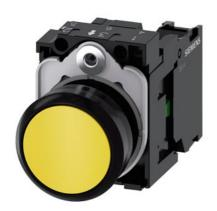
Pushbutton, 22 mm, round, plastic, yellow, pushbutton, flat, momentary contact type, with holder 1 NO, screw terminal, with laser labeling, lower case
