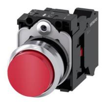
Pushbutton, 22 mm, round, metal, shiny, red, pushbutton, raised, momentary contact type, with holder, 1 NC, spring-type terminal, Z=20-unit packaging
