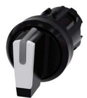
Selector switch, illuminable, 22 mm, round, plastic, white, selector switch, short, 3 switch positions I-O-II, latching, actuating angle 2x45°, 10:30h/12h/13:30h, with laser labeling, inscription or symbol Customer-specific selection with SIRIUS ACT configurator (CIN)
