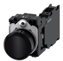
Pushbutton, 22 mm, round, plastic, black, pushbutton, flat, momentary contact type, with holder 1 NO+1 NC, spring-type terminal, with laser labeling, upper case and lower case, always upper case at beginning of line
