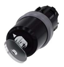
key-operated switch Siemens, 22 mm, round, plastic with metal front ring, lock number SSG10, with 2 keys, 2 switch positions O-I, latching, actuating angle 90°, 10:30h/13:30h, key removal O+I, with laser labeling, upper case and lower case, always upper case at beginning of line
