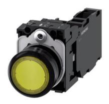
Illuminated pushbutton, 22 mm, round, plastic, yellow, pushbutton, flat, momentary contact type, with holder, 1 NO+1 NC, LED module with integrated LED 110 V AC, screw terminal, with laser labeling, inscription or symbol Customer-specific selection with SIRIUS ACT configurator (CIN)
