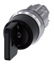
Key-operated switch O.M.R, 22 mm, round, metal, shiny, lock number 73034, black, with 2 keys, 3 switch positions I>O<II, momentary contact type, actuating angle  $2x45^{\circ}$ , 10:30h/12h/13:30h, key removal O, with laser labeling, lower case
