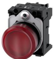
Indicator lights, 22 mm, round, plastic, red, lens, smooth, with holder, LED module with integrated LED 110 V AC, screw terminal, with laser labeling, lower case
